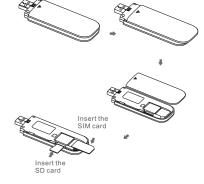
When install the SIM and SD card, please open the back of the device and remove it, put the Micro-SIM card and SD card into the slot according to the direction of the arrow. After installation successfully, put the cover back on the device and close it.
